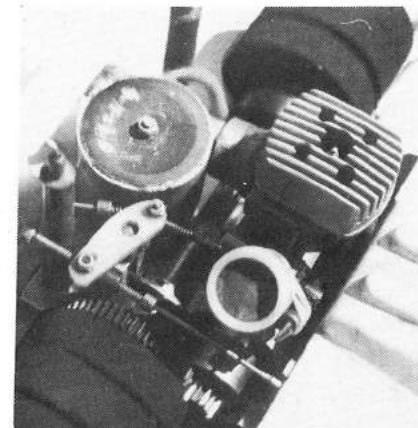
Dustbin silencer, "big head" heat sink, carburettor filter and springloaded servo saver linkage to disc brake.
